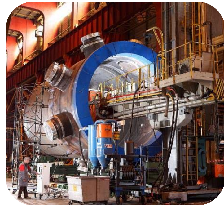
Reactor Pressure Vessel – St-Marcel
