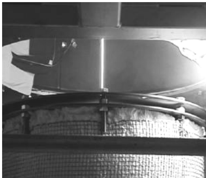
Figure 2.17. Glass pouring in La Hague R7 facility (Source: COGEMA – France)
