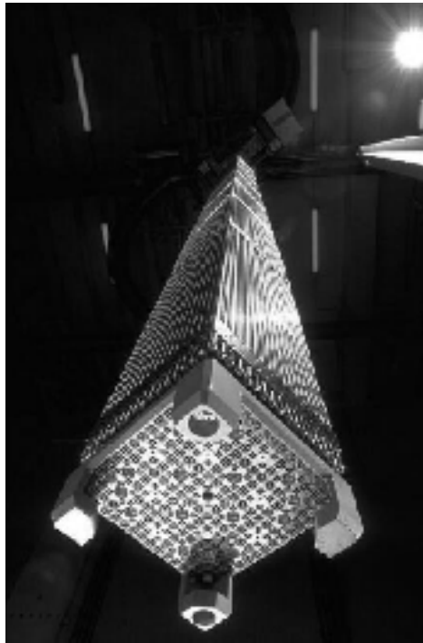
Figure 2.2. View of a typical PWR fuel assembly (Source: COGEMA – France)
