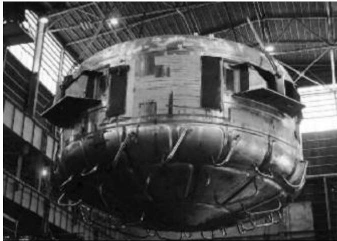
Figure 8.5. HLLW tank showing bottom cooling jackets (Source: Japan)
