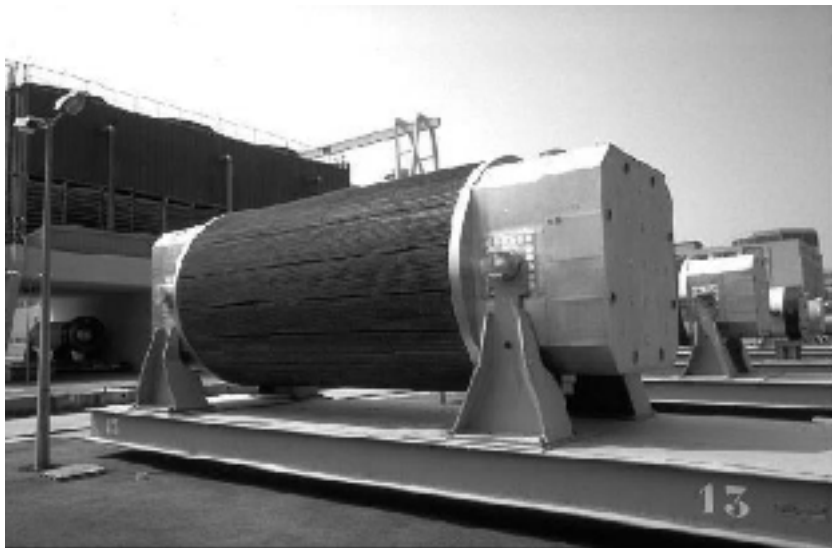
Figure 11.1. Typical type B package (Source COGEMA – France)
