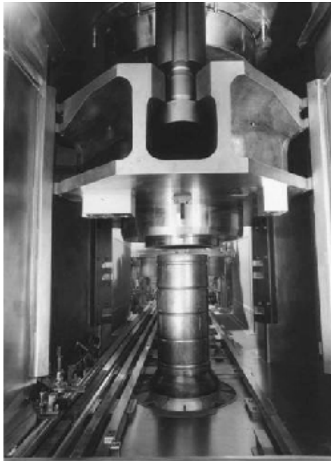
Figure 8.1. Compacting press in the ACC facility at La Hague (Source: COGEMA – France)
