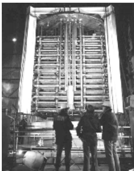
Figure 8.4. View of an HLLW tank with cooling coils (Source: BNFL – United Kingdom)
