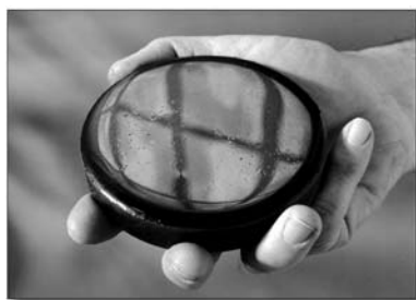
Test glass produced by vitrification process.
