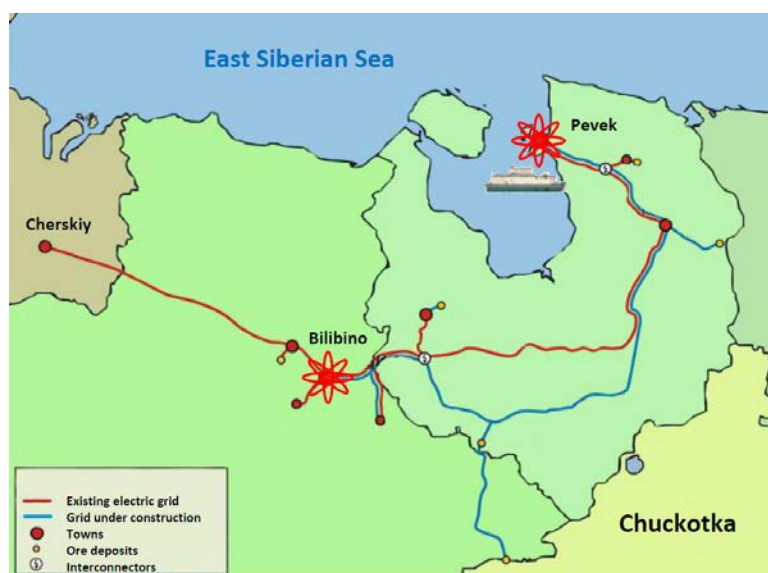
Figure 6.4: Chaun-Bilibino power grid
