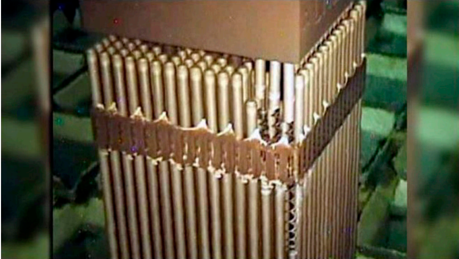
FIG. 9. Fuel damage / baffle jetting.
