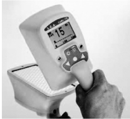
Figure 4.3 The contamination monitor CoMo 170 by S.E.A. 4 with plastic scintillator
