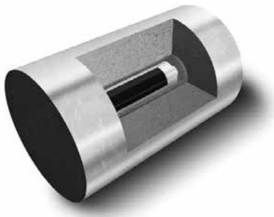
Figure 2: Artist's impression of OPERA supercontainer for heat-generating HLW
