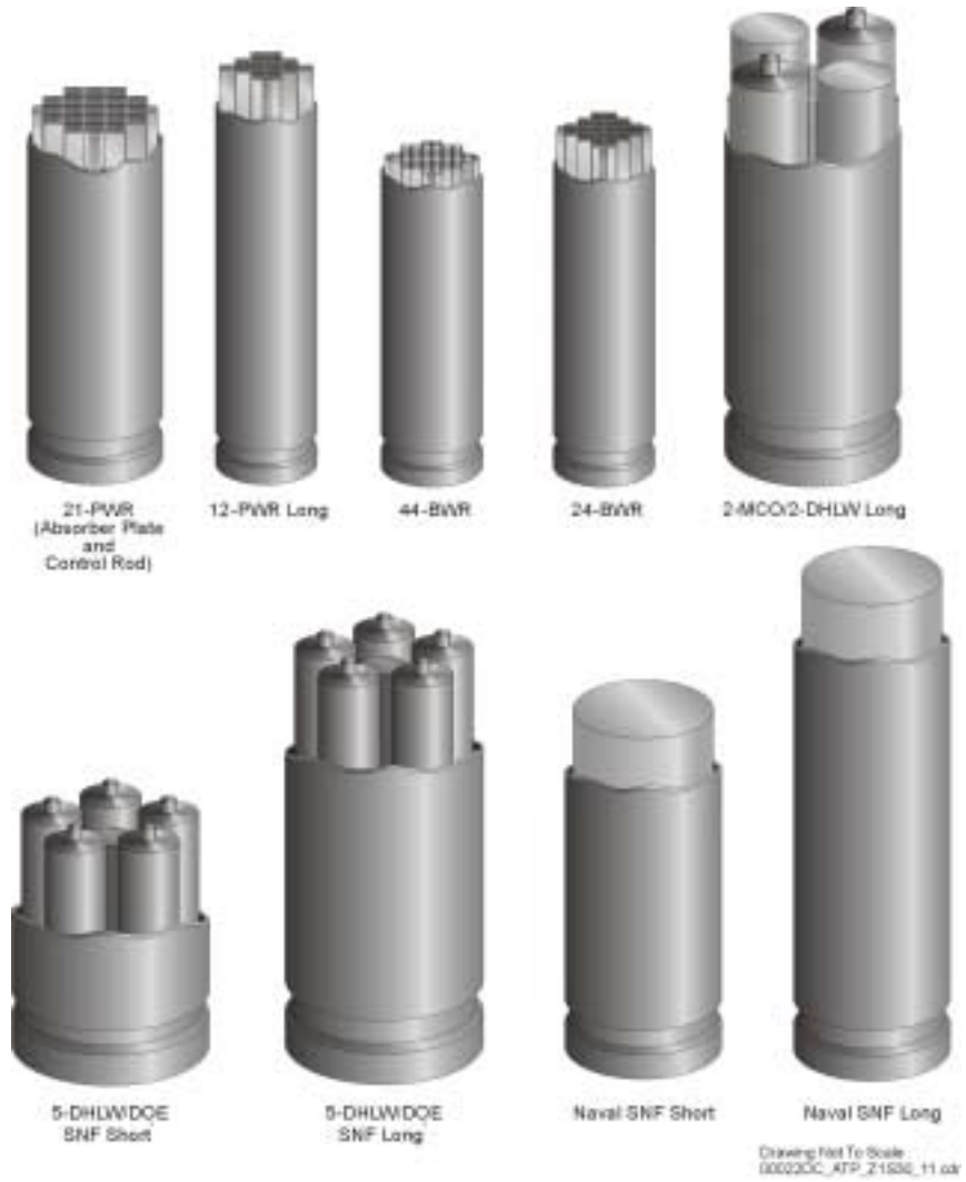
Figure 7. Waste Package Designs with Waste Forms
