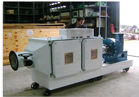
New portable filtration unit.
