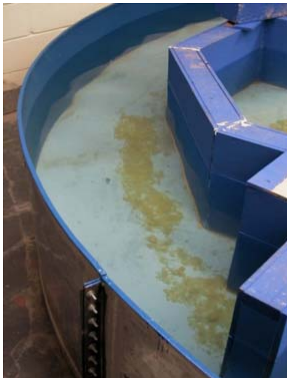
Figure 4-11: Debris Stalled in a Slow-Flowing Region of the Simulated Annulus
