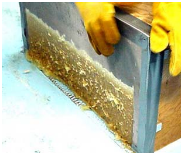
Figure 4-12: Typical Accumulation of Fine Fibrous Debris
