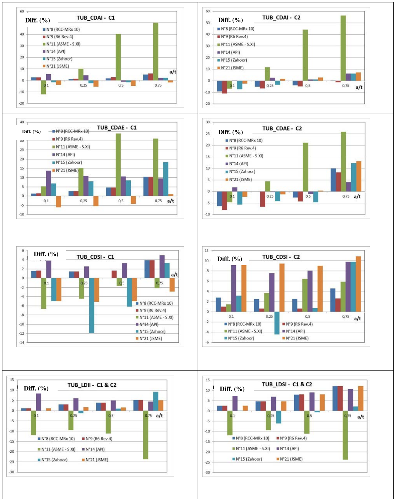
Figure 7: Percentage of differences compared to FE reference solution obtained by different codes application
