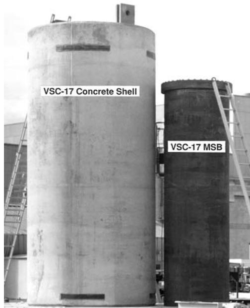
Figure 11.9 Photo of the concrete shell and sealed canister
