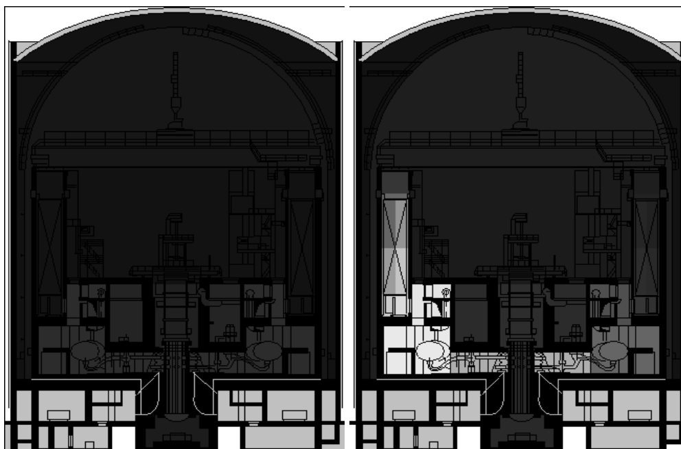
Fig. 4.1-4 Temperature distribution in Loviisa NPP ice condenser containment at 0 s (left) and 3 s, (right) after a 500 cm 2 break in cold leg calculated by APROS SA. (Color gradient is from blue to red to yellow with blue corresponding 20 °C, red 60 °C and yellow 100 °C) [1]
