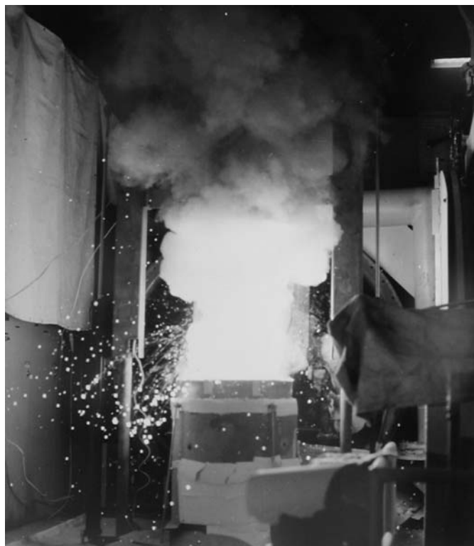
Fig. 3.9-1 Photograph of a high temperature melt interacting with calcareous concrete and the associated aerosol production
