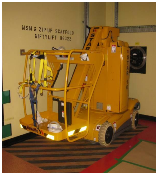
Phase 2 – Mobile access platform
